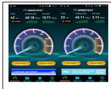
Fig. 6. Measurements of bandwidth and latency using the Speedtest application on Google Android devices connected to IPaccess eNB equipment, as described in the setup of Testbed 1 at 5GIC Surrey.
